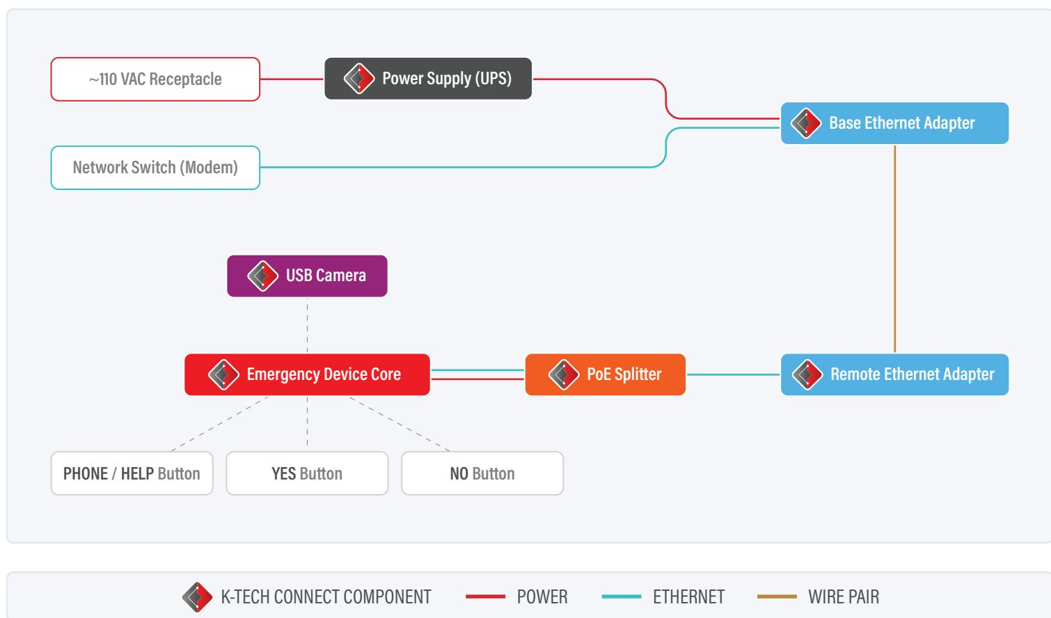
K-Tech Connect Emergency Devices are meant to work alongside the elevator's emergency phone, adding live video and text communication, while still relying on standard voice communication.
